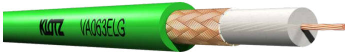
75 Ohm - analog video patch kabel 0.6L/3.7 - economic - PVC • flexibler innenleiter (7 x 0,20 mm)
